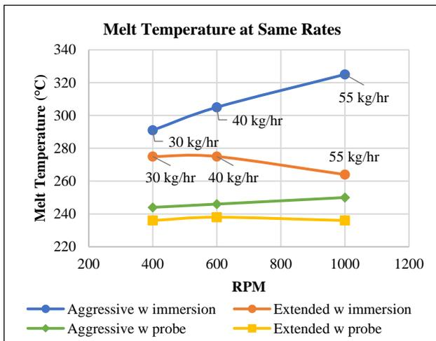
Figure 6: Comparing the melt temperature at same rates with the flush and immersion melt probes.
