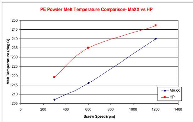
Figure 3: Melt temperature comparison: MAXX vs HP for 12 MFI PE powder.
