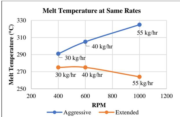
Figure 5: Comparing the melt temperature at the same rates.
