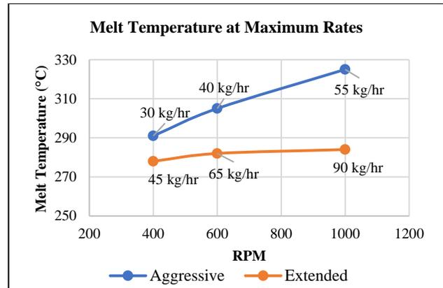
Figure 7: Comparing melt temperature at maximum rates.
