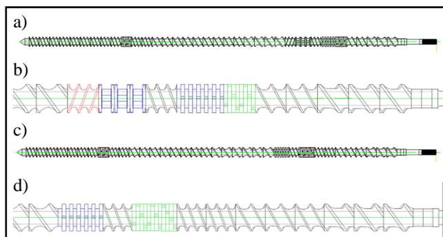
Figure 4: a) Aggressive melting zone screw design b) Aggressive melting zone closeup c) Extended melting zone Screw design d) Extended melting zone closeup.
