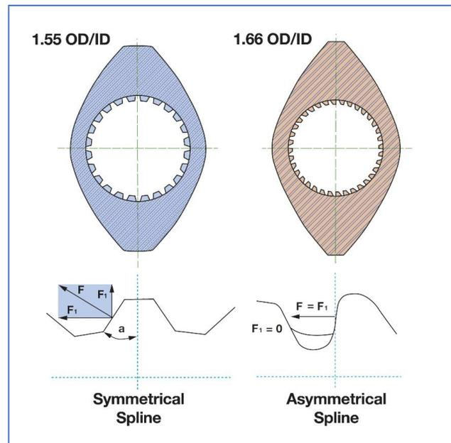
Figure 1: End view HP and MAXX screw element geometries.
