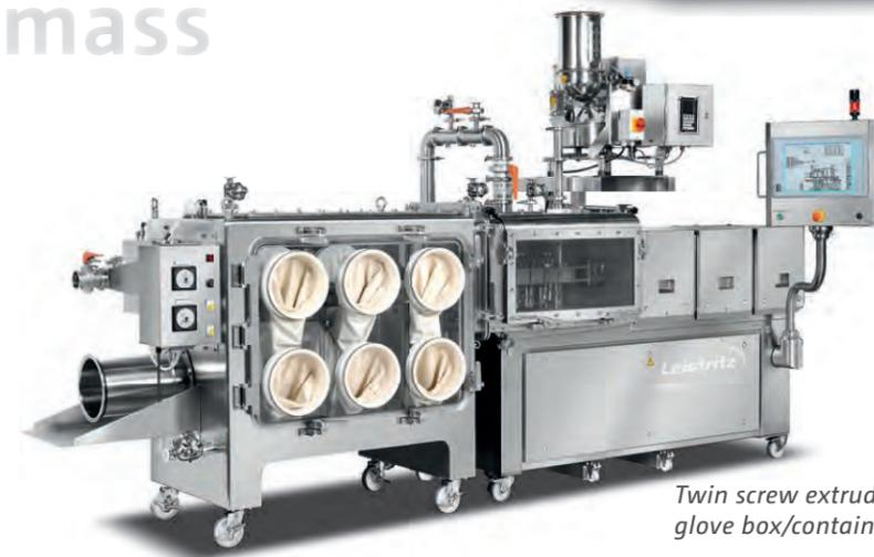
Twin screw extruder with glove box/containment features
