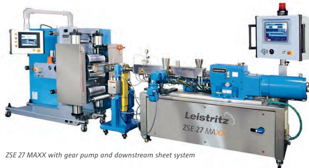
ZSE 27 MAXX with gear pump and downstream sheet system
