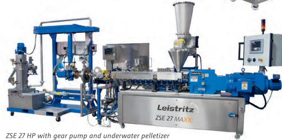
ZSE 27 HP with gear pump and underwater pelletizer
