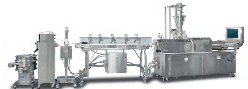
ZSE 27 micro-pelletizing system with in-line gauge, pelletizer and classifier
