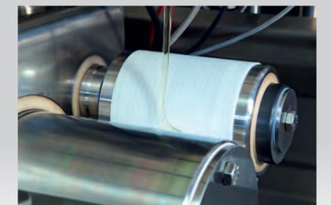
ZSE 18 HP-PH extruding to the chill roll
