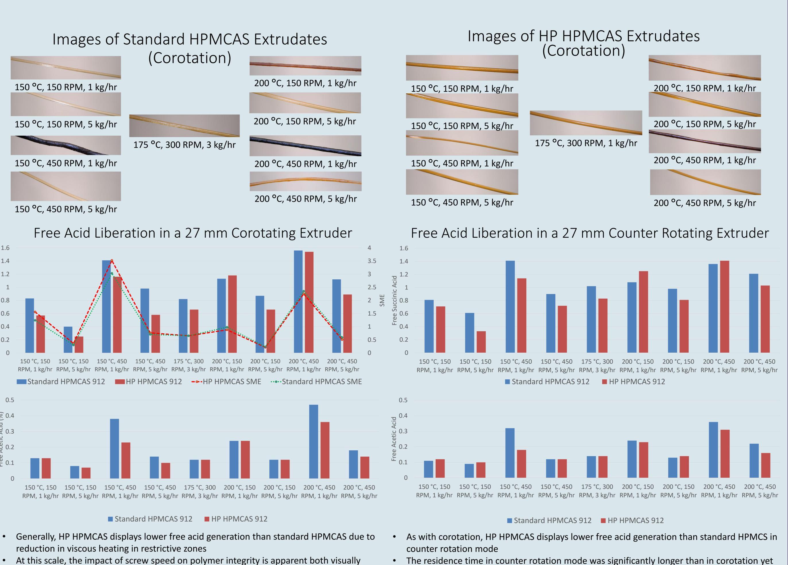
and by high free acid levels; this is a crucial process parameter to consider upon scaling • The primary free acid contributor is succinic acid (boiling point of acetic acid is 118 °C) • At high temperatures, proper control of feed rate and screw speed enables successful extrusion of both grades with acceptable acid levels (< 1% total free acids)
