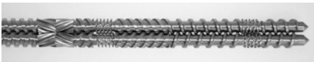
Figure 5c. Hexa-lobal mixing, degassing, thermal homogenization and discharge.
