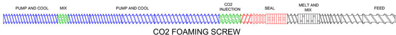
TSE screw schematic denoting unit operations for injection of physical blowing agents
