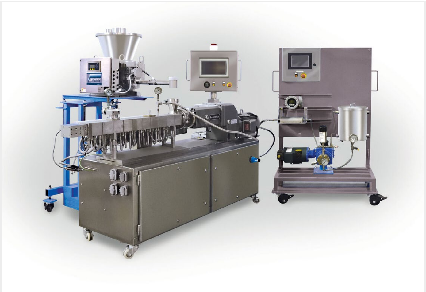
Example twin screw extruder with solids and liquid metering equipment
