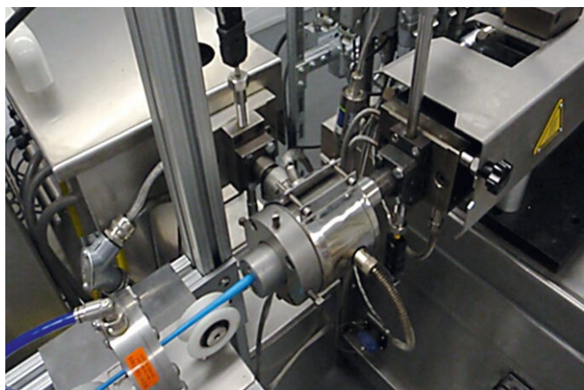
Co-extruded rod/ tube being developed in the Leistritz Process Lab
