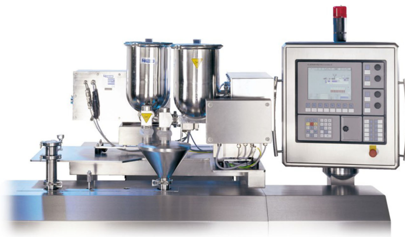
Fig. 16. Setup of multiple loss-in-weight feeders to meter excipients and APIs into a TSE
