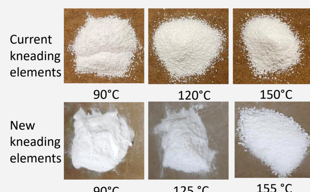
Fig. 6. Visual images showcasing granulation with current kneading elements (5 mm disc width and 0.1 mm overflight clearance) staggered at 30° vs no granulation until 155 °C with new kneading elements staggered at 30°
