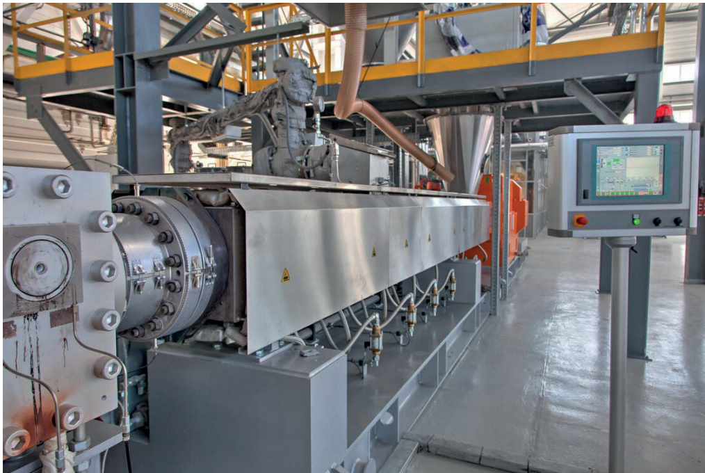
Heated/insulated vent stack attached to ZSE MAXX process section
