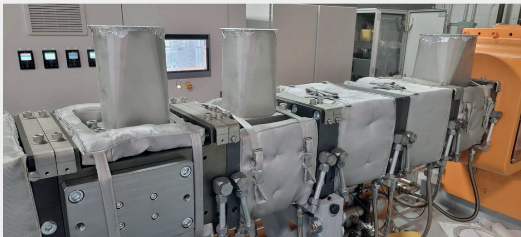
ZSE MAXX barrels with insulation blankets
