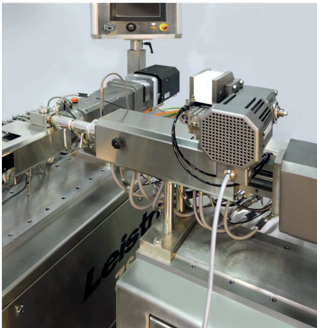
Tandem extrusion: Counter-rotating TSE mated to co-rotating TSE
