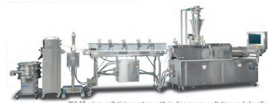
ZSE 27 micro-pelletizing system with in-line gauge, pelletizer and classifier
