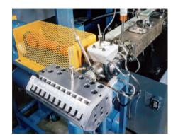
Gear pump and sheet die
