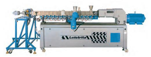
Micro-27 @ 60/1 L/D configured for compounding and foam profile extrusion
