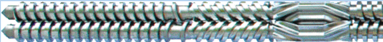
Co-rotating and counter-rotating twin screw sets.
