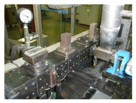
ZSE-27 MAXX process section used for test
