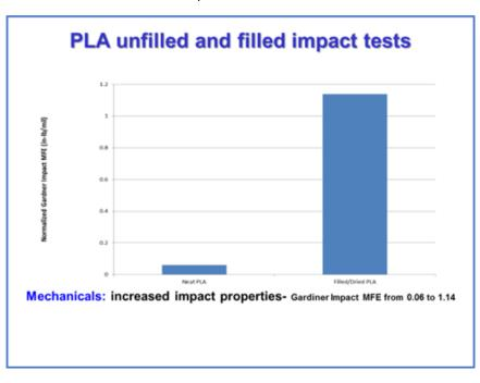
**Processing undried PLA pellets and regrind:** Undried PLA pellets (50%) and edge-trim (50%) with residual moisture levels between 1500 and 3000 ppm were metered into a ZSE-50 MAXX TSE with a process section designed to optimize venting efficiencies for removal of the moisture. The process was developed and the test was performed at 200 kgs/hr and 250 rpms. The TSE process section design and results the molecular weight loss (approx. 7%) for the dried and undried samples are indicated below.
