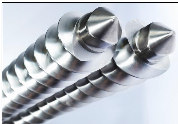
TSE technology: 2-screws interact with each other
