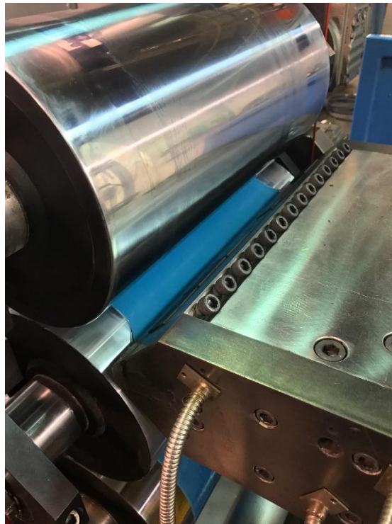
Draw down effect between die and take-off roll
