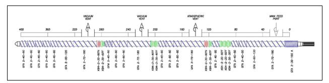
Figure 7: ZSE-50 MAXX screw/process section design
