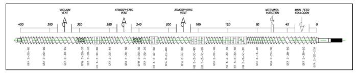
Figure 5: ZSE-27 MAXX screw/process section design
