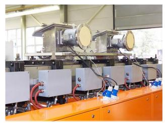
Figure 9: Heated vent stack
