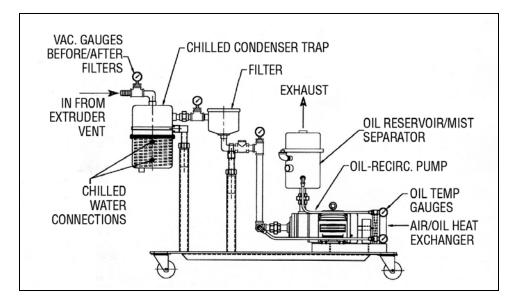
Figure 11: Example of vacuum venting system components
