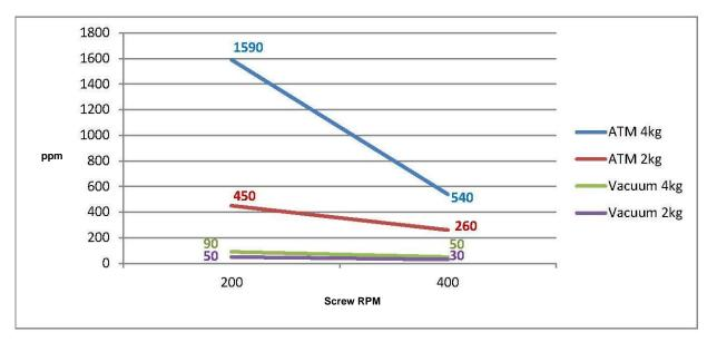
Figure 6: Residual solvent (in PPM) for various operating conditions
