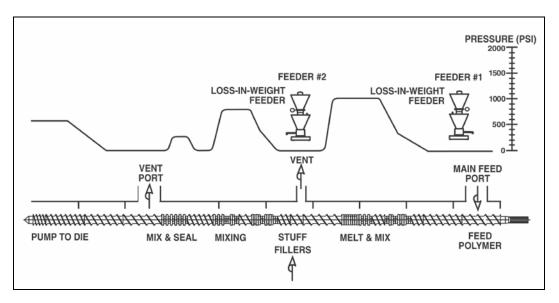
Figure 2: Pressure gradient in a starve fed twin screw extruder
