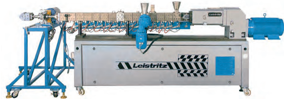
Micro-27 @ 60/1 L/D configured for compounding and foam profile extrusion
