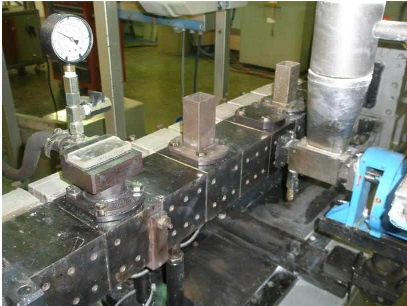
ZSE-27 MAXX process section used for test
