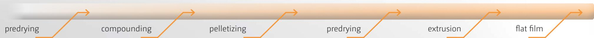
**Direct extrusion (single-stage): raw material → film**
