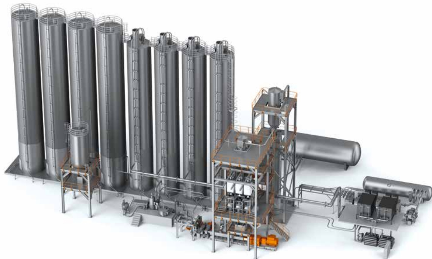
Example of a major project: 3D visualization of a compounding line for stabilizing PP powder directly after polymerisation
