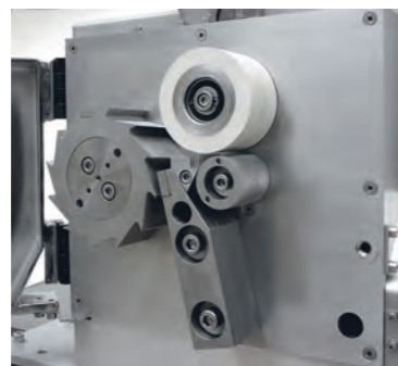
Leistritz ZSE 18 HP-PH with cooling conveyer belt and strand pelletizer for the production of cylindrical pellets
